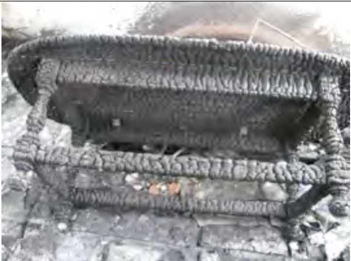
Photo 22: Low burning and burn patterns to underside of wooden table in burn cell #4.
