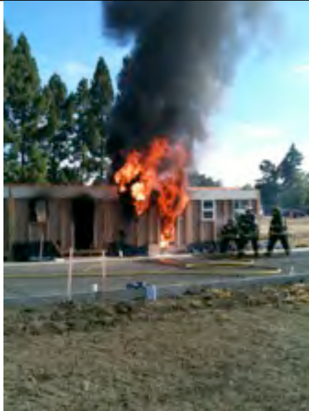
Photo 3.3: Burn Cell 3 during flashover
