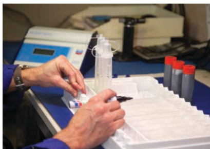
2. Prepare the samples using the DispoRack and ITUs.
