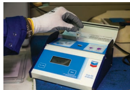
3. Test the prepared samples using the Drip Oil Analyzer.
